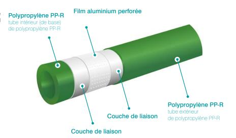
Construction du tube composite KAN-therm PP Glass
