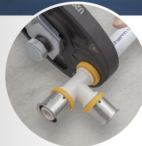
05 | Starting the press drive and pressing the joint.
